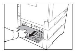
**NOTE:** If the paper cannot be removed, do not try to forcefully remove it. Go to paper jam in the feed unit on page 10-19.
